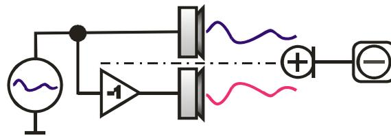
Figure 3: Scheme of the basic principle of ANR
