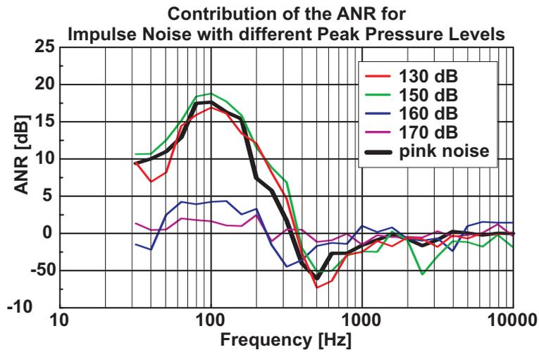
Figure 21: Contribution of the ANR for impulse noise (explosion) with different peak pressure levels and for continuous noise.
