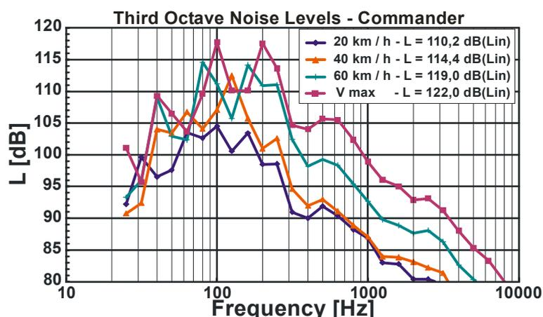
**Figure 1:** Typical noise inside an armoured vehicle
