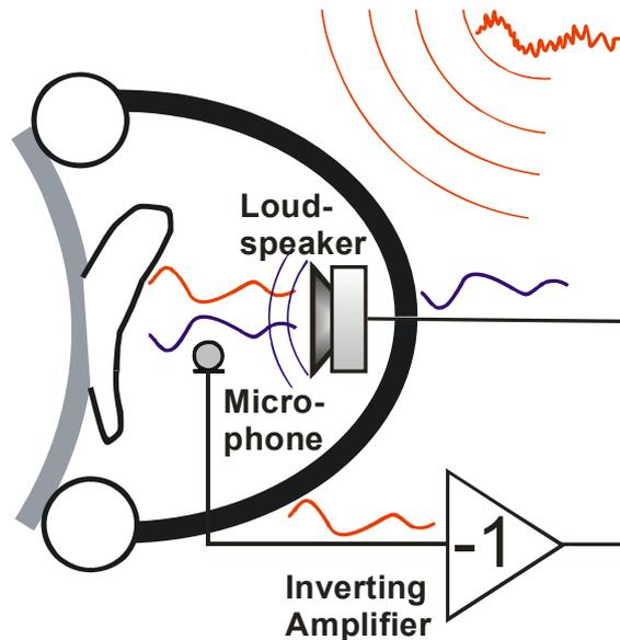
Figure 6: Basic principle of ANR using feedback control
