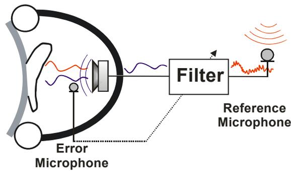
Figure 5: Principle of a feed forward control
