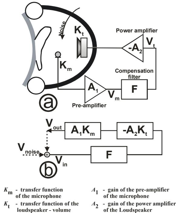
**Figure 7:** (a) Different electrical and electro-acoustical elements of the ANR system.
