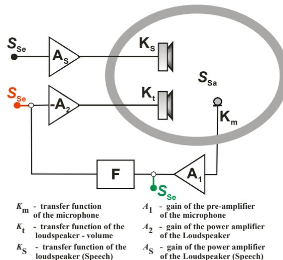
**Figure 8:** Insertion of a communication signal into an ANR system
