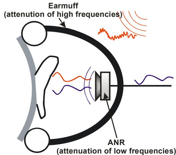
Figure 4: Principle of ANR underneath an earmuff
